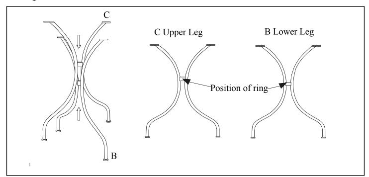
Correctly identify each Leg components(B and C) by the position of ring. Position and insert Upper Leg Assembly (C) into Lower Leg Assembly (B) as shown.
