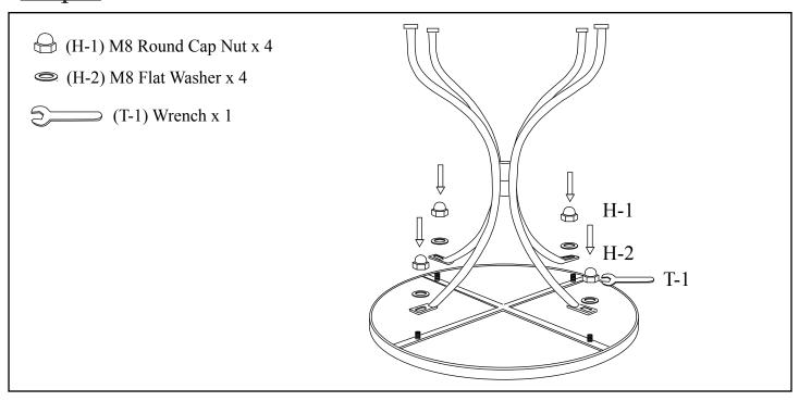
Position and insert Leg Assembly (B and C) tabs onto the four mounted threaded studs on Table Top underside. Secure Legs Assembly onto Table Top using Flat Washers(H-2) and Round Cap Nuts(H-1) stacking the hardware in the order as shown. Tighten all nuts using Wrench(T-1) provided.
